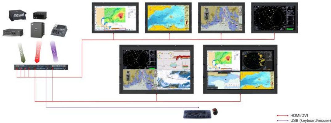
Pacific MS-1 with eight source inputs and one workstation with two quad-view outputs and four single-view outputs
